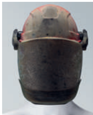
According to 7 kA short circuit electric arc
